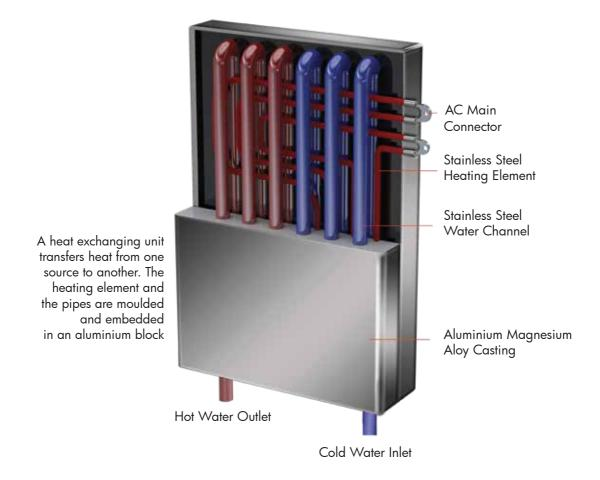
The water enters and circulates through the pipes and gets heated by the heating element using a quick transfer of heat through the aluminium block to the water in the pipes. This technology gives instantaneous water, without direct contact between the heating element and water. This in turn increases energy efficiency, lowers operating costs and ensures total safety. It avoids scale formation and recurring maintenance in hard water areas.
